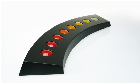
The ability to print 500,000 colors make lighting prototypes almost identical to the real thing.
