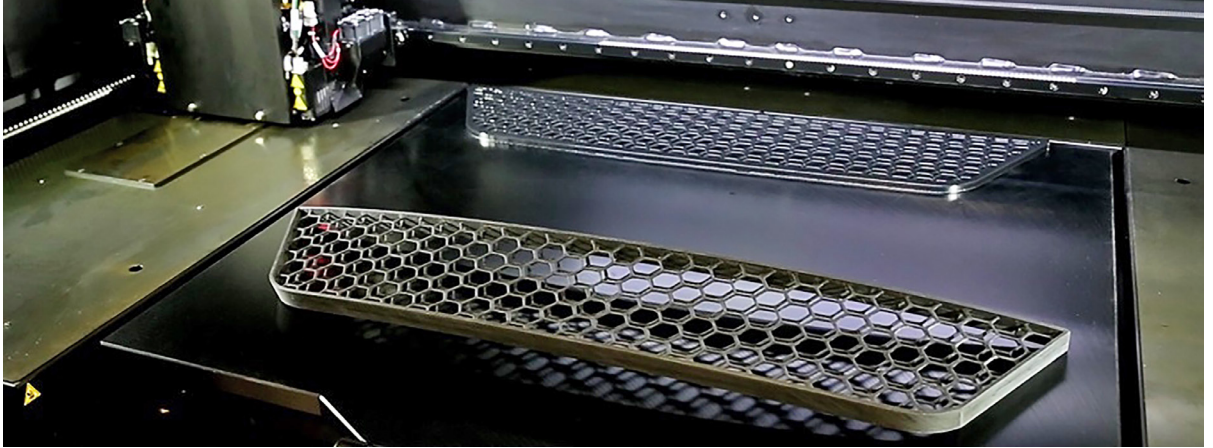
A grating for a car example, 3D printed in one piece.
