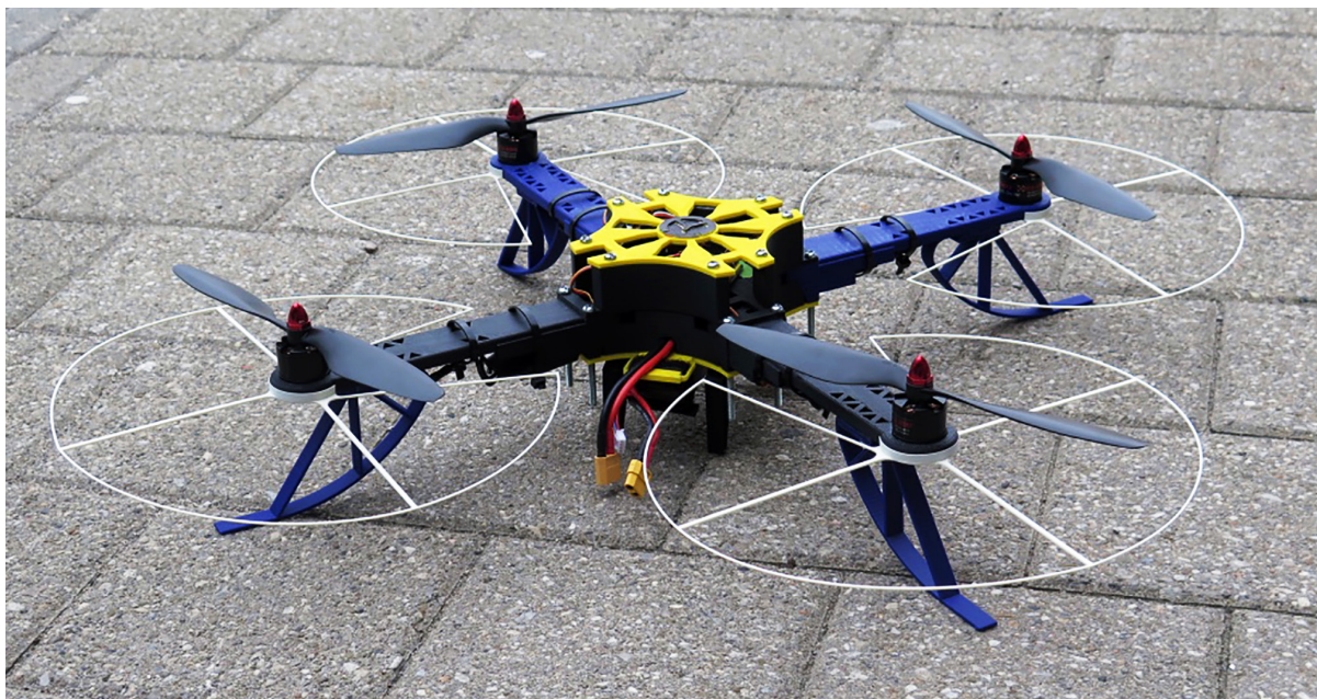
This 3D printed drone quadcopter is the result of a design challenge given to students at the John Paul II Catholic Secondary School in London, Ontario, Canada.
