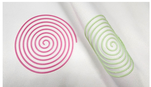
Figure 8: Flexible material thin continuous line – example
