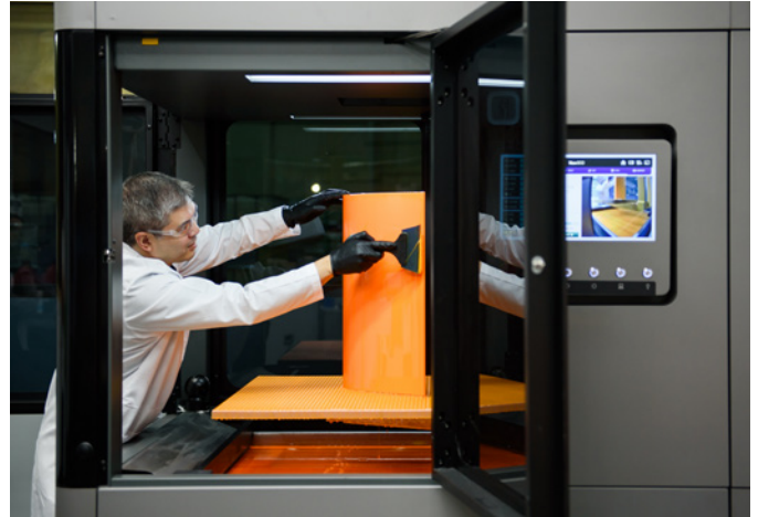
The Neo 800 is big enough to print the large airfoil models Gulf Wind Technology needs for wind tunnel testing.
